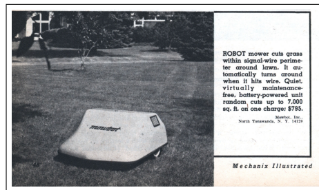
Fig. I.1: Mowbot, the first mobile robot in home automation
