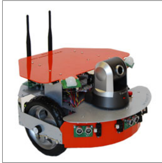
Fig. 1.8: Mobile robot equipped with a camera
